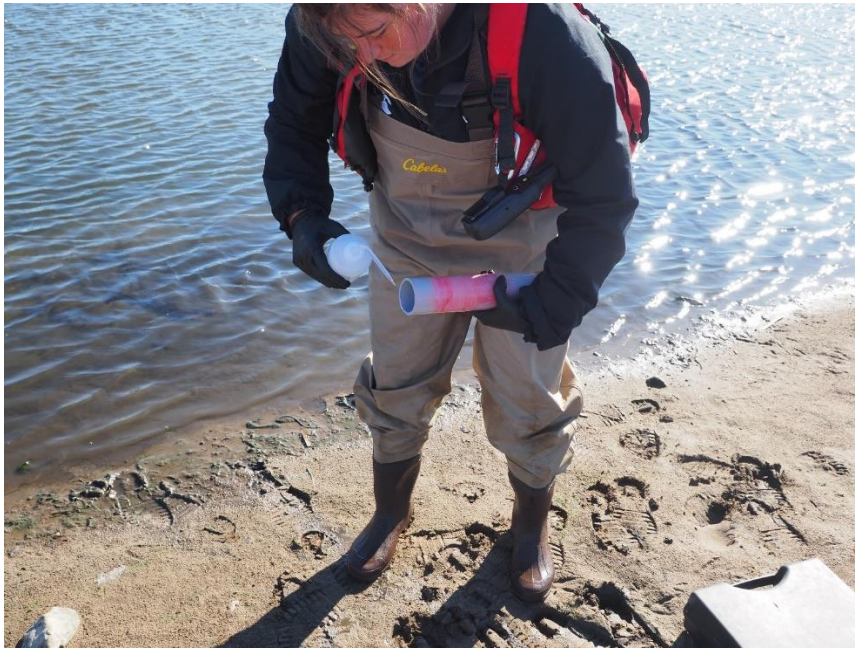
Figure 3. ACAP staff member cleaning a plastic corer after collecting a sediment sample.
