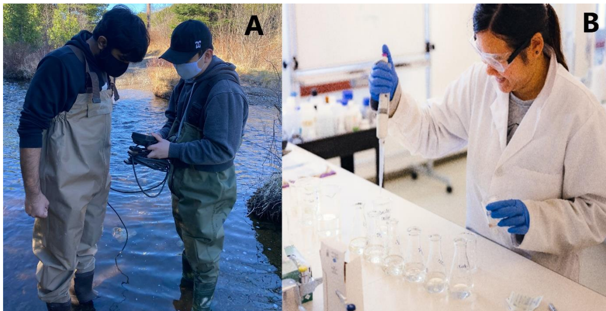
Figure 2. Water quality sampling and analysis methods. (A) Staff collecting data in-situ using a YSI Pro Meter Plus; (B) NBCC Chemical Technology student analyzing samples for ammonia using an alternate method.
