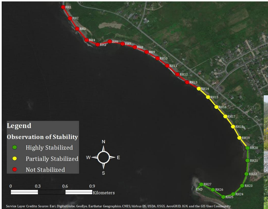
Figure 18: Stability of Red Head observed in summer 2021. Images: Top left, majority of the coastline are steep slopes that are not stabilized. Bottom left, overhanging vegetation is observed.
