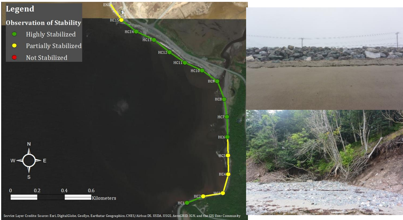
Figure 23: Observation of stability at Hazen Creek in summer 2021. Images: Top right, riprap and powerlines observed in HC13. Bottom right, trees falling from slopes in HC6. Both images show the highwater mark, resulting in a reduced backshore along the coastline.
