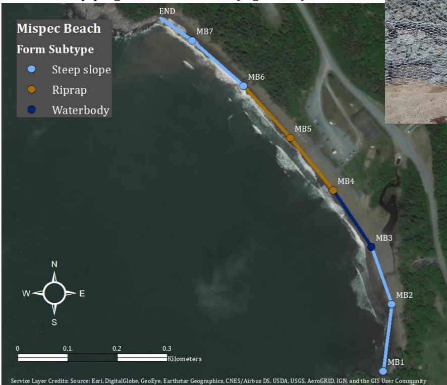
Figure 11: Left, form types along Mispéc Beach observed summer 2021. Image above, showing a drainage channel in the riprap where repairs may be required.
