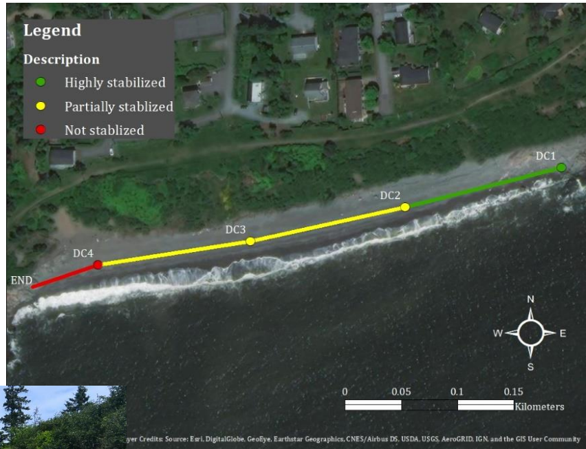
Figure 32: Observation of stability at Duck Cove summer 2021. Image left: Eroded section at DC4 where coastline is not stabilized and sand is the predominant soil texture. Staircase access is on the left where vegetation returns but erosion is observed around the access point.
