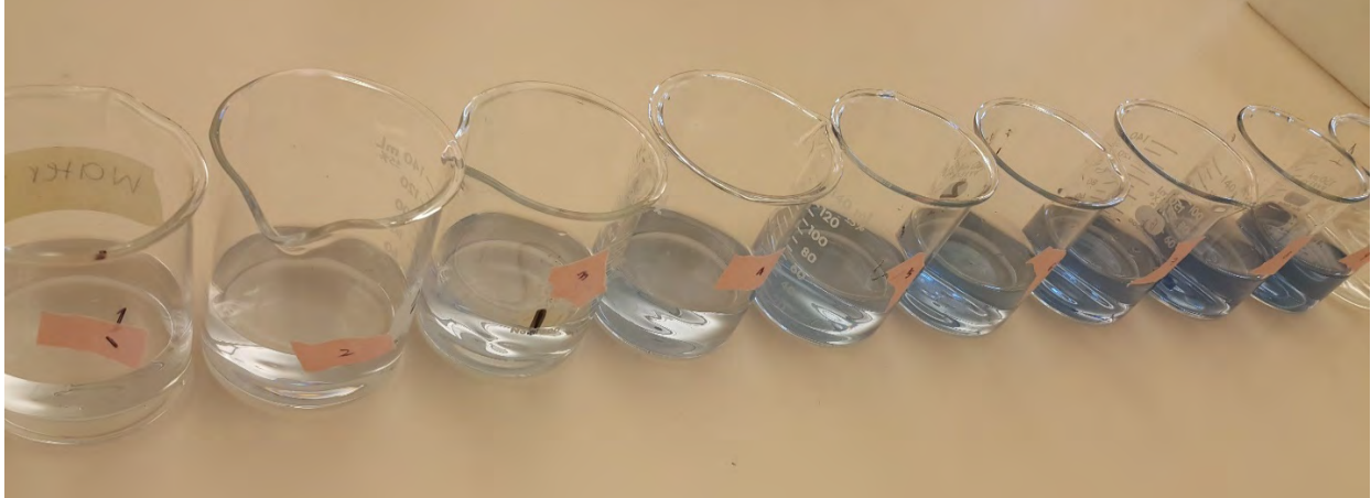
Figure 13. The colour development of standards for the orthophosphate calibration curve.
