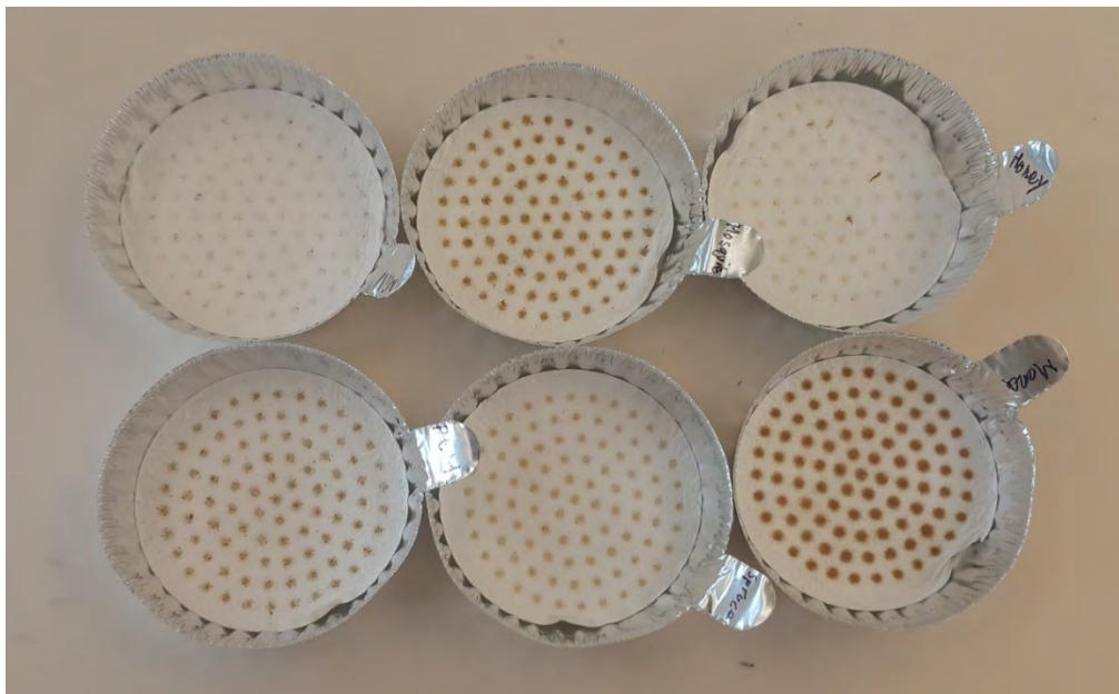
Figure 14. Image showing solids left on filter paper after filtration was completed using the Total Suspended Solids procedure.
