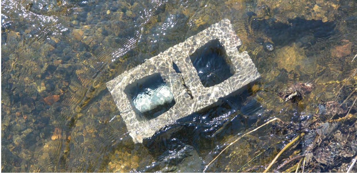
Figure 17. Example of temperature logger attached to a cinder block. All cinder blocks were covered underwater.
