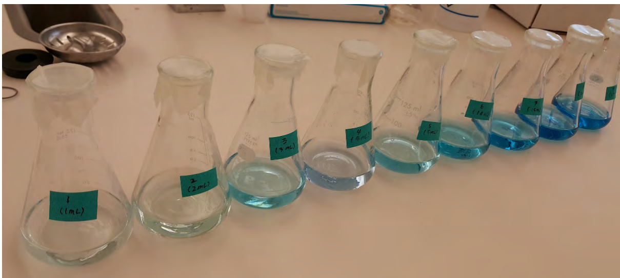
Figure 16. The colour development of standards for the Ammonia calibration curve.
