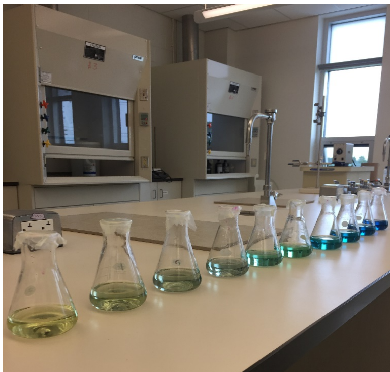
Figure 2.3.D: Photograph showing the colour development of standards for the Ammonia calibration curve.
