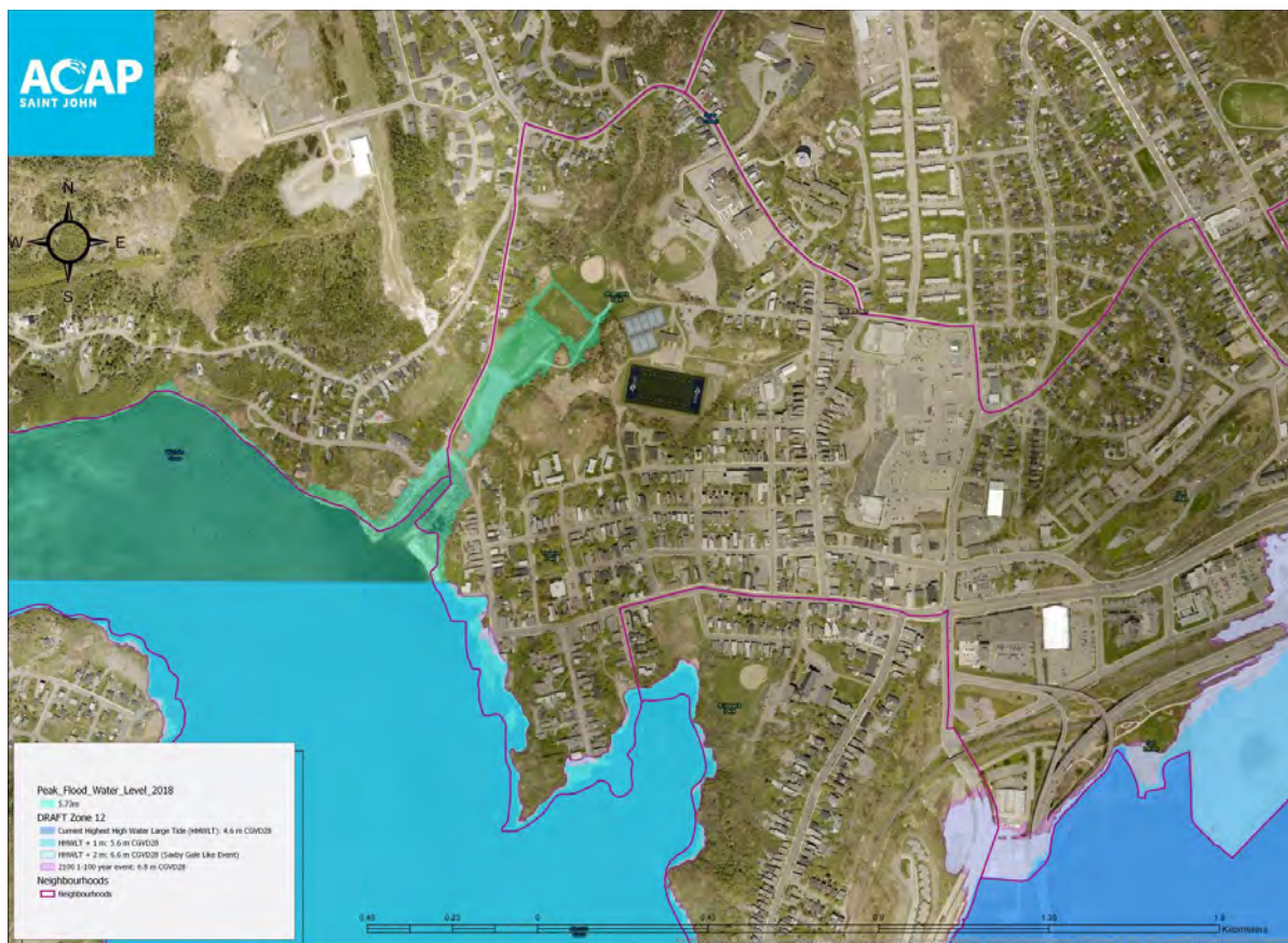
Figure 26: Coastal hazard flood map showing flooding levels in the North End, Saint John, NB.
