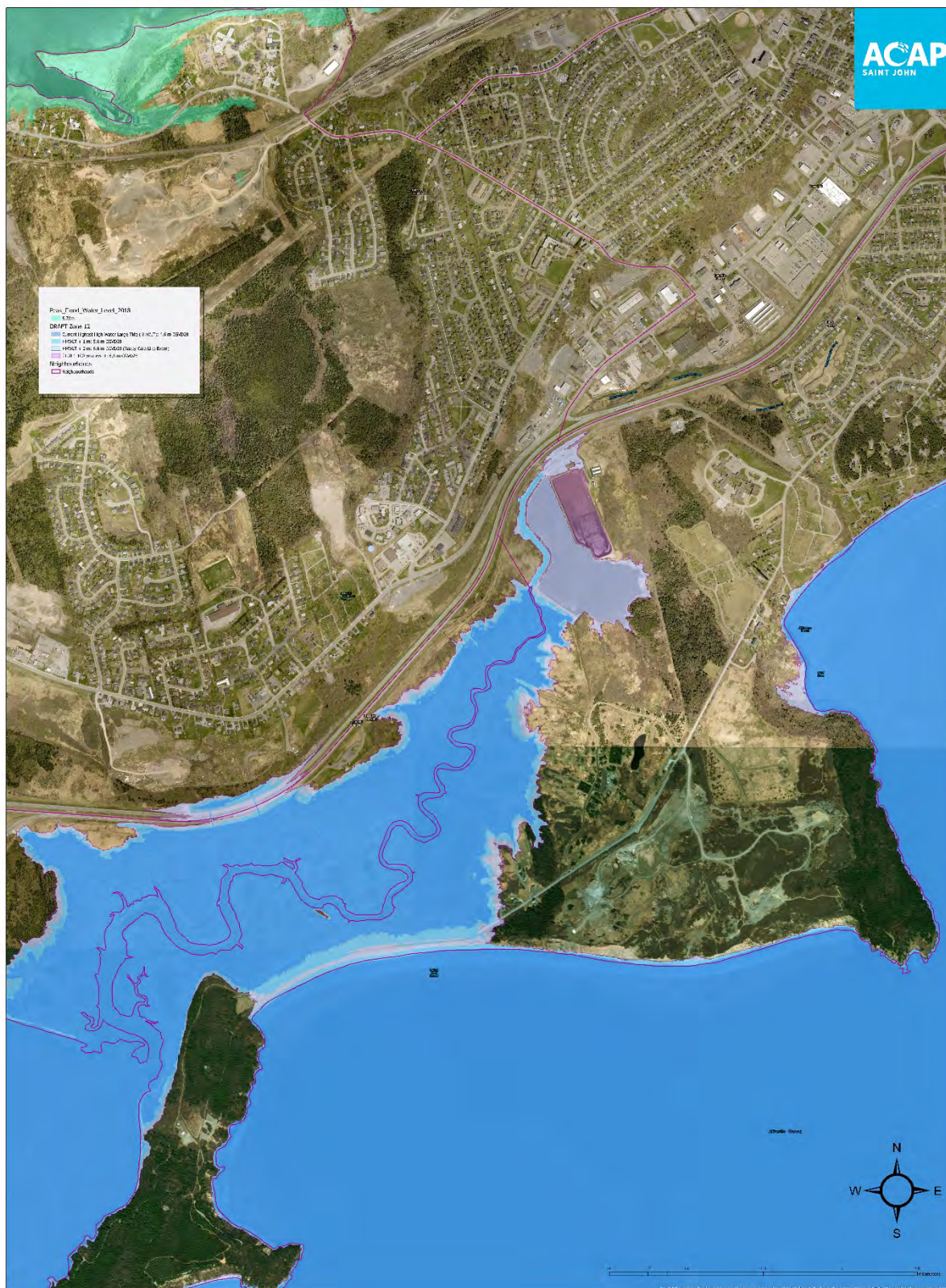
Figure 31: Coastal hazard flood map showing flooding levels in the West Side and Saint Rest's Marsh, Saint John, NB.
