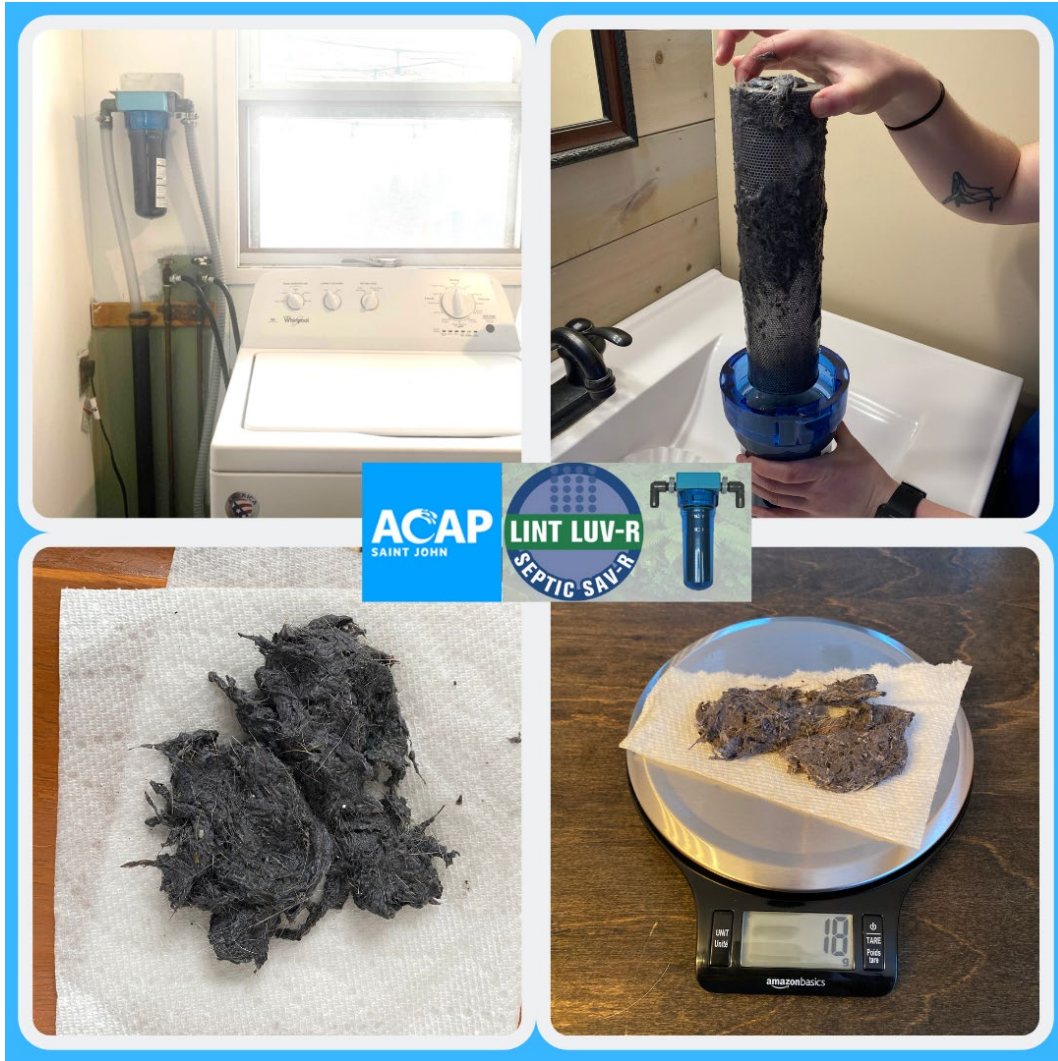
Figure 11. Images that show the process of lint collection, drying, and weighing.
