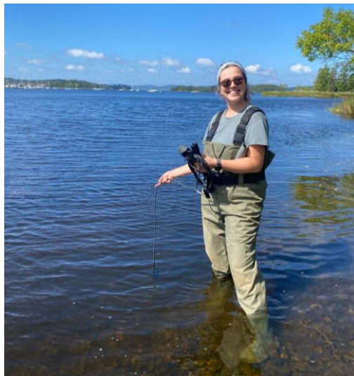
Figure 2. ACAP Saint John field technician deploying a YSI multimeter to collect in-situ water quality parameters.
