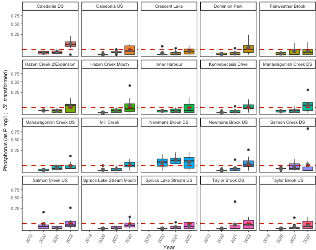
Figure 19. Orthophosphate concentrations (mg/L) as P across sites in the Greater Saint John area between 2019 and 2022. The mean values for each site are represented by grey dots, the outliers are represented by black dots, and the chosen threshold value (0.04 mg/L) is represented by the dotted line.
